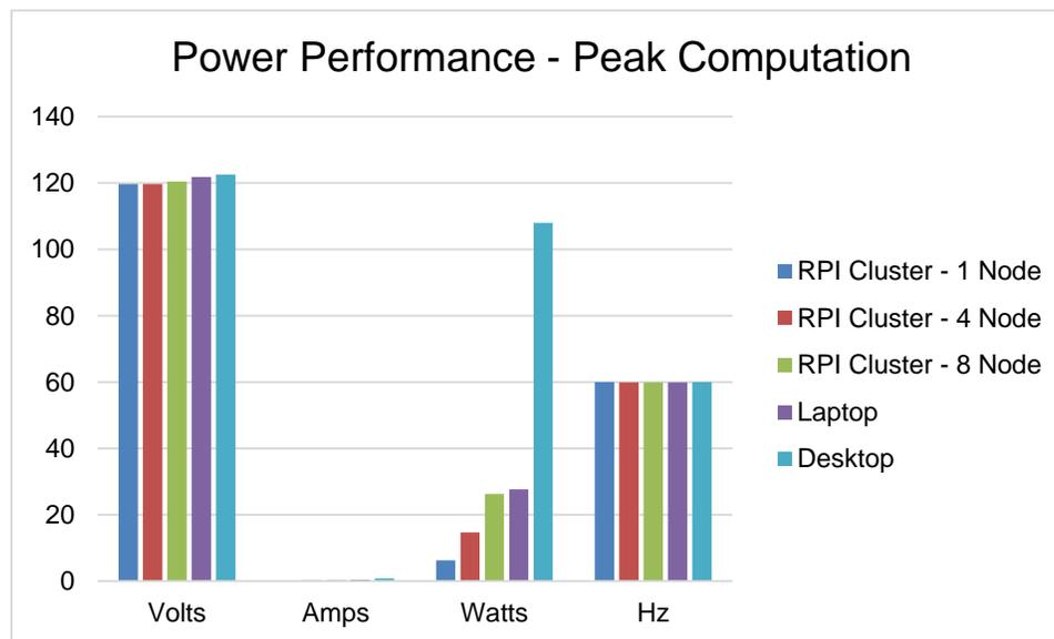
**Figure 9: Results for Machines At Peak Computation**
